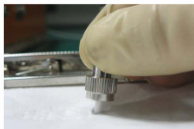
Figure 5-96 Cleaning optical fibers with special cleaning tissues
