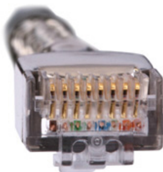
Figure 5-33 Contact strips of the same height
