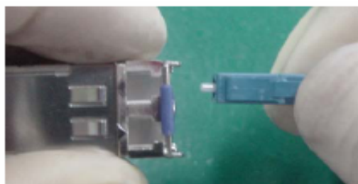
Figure 5-98 Using fibers to protect an optical module
