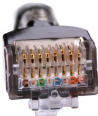
Figure 5-32 Contact strips of different heights
