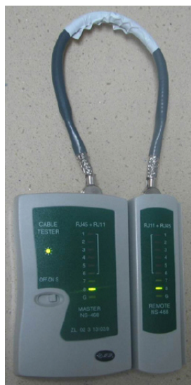
Figure 5-39 Testing the conduction and connections of wires
