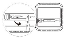
3 Insert the SIM card gently into the SIM card slot in the direction shown in the figure below until it clicks. Then close the SIM card cover.
