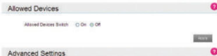
4. After open the whitelist function, you need to know the user client's MAC address and add to the list, the format is XX:XX:XX:XX:XX:XX. You can add up to 10 devices if they are all going to connect, because the Wi-Fi chip can only support 10 devices connected at the same time.
