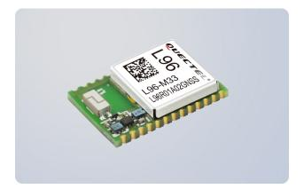
L96 is a concurrent multi-GNSS receiver module with embedded chip antenna. With 33 tracking channels, 99 acquisition channels and 210 PRN channels, L96 supports concurrent reception of up to three GNSS systems (GPS+GLONASS+Galileo). The built-in LNA provides the module with better performance under weak signal areas. The embedded chip antenna reduces the total size of customers' applications. To meet varied application demands, L96 also provides an external antenna interface.
