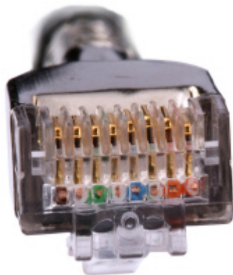
Figure 5-32 Contact strips of different heights
