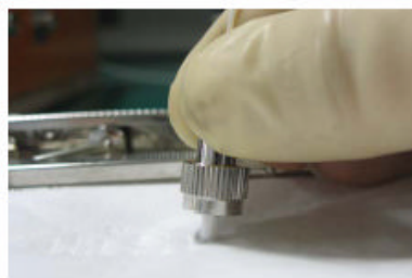
Figure 5-96 Cleaning optical fibers with special cleaning tissues
