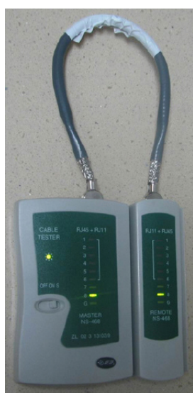
Figure 5-39 Testing the conduction and connections of wires
