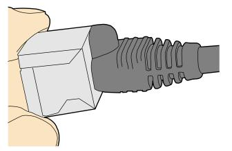
**Step 4** To remove an Ethernet connector, press the locking key and pull out the connector, as shown in Figure 5-53.
