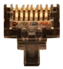
**Step 5** Hold the connector with the side facing towards you, and check whether you can see the cross-sections of the wires. Ensure that the ends of the wires are in good contact with the edge of the RJ45, and that the contact strip blade extends beyond the ends of the wires and is crimped with the wires. If not, replace the connector. Figure 5-37 shows an unqualified piece.
