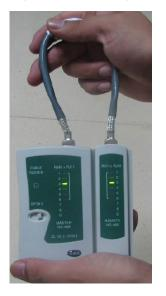
The procedure for testing a crossover cable is the same as that for testing a straight-through cable except for the sequence in which the indicators turn on. You need to refer to the wire connections of a crossover cable.
