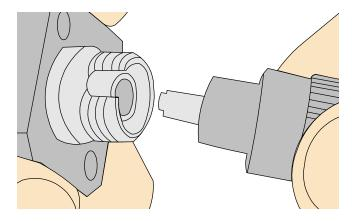
**Step 3** Align the male connector with the female connector and gently push the male connector until it is completely seated in the female connector, as shown in Figure 5-59.
