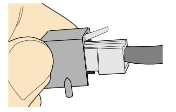
**Step 4** To remove an Ethernet connector, press the locking key and pull out the connector, as shown in Figure 5-57.
