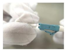
4. If a receptacle or an optical connector has not been used for a long time and is not covered with a protective cap, you need to clean it before using it. Clean a receptacle with a cotton swab, as shown in Figure 5-100. Clean an optical connector with cleaning tissues.
