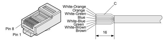
Table 5-6 Connections between wires and pins (using a straight-through cable as an example)
