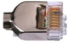
**Step 4** Check whether the contact strips and the plastic separators are well aligned and intact. If a separator is skew and cannot be fixed, replace it with a new RJ45 connector. Figure 5-36 shows an unqualified piece.
