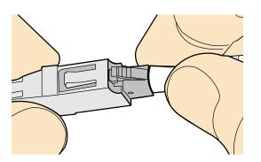
**Step 5** To disassemble an LC fiber connector, press the locking nut to release the locking clips from the bore, and gently pull the male connector, as shown in Figure 5-65.
