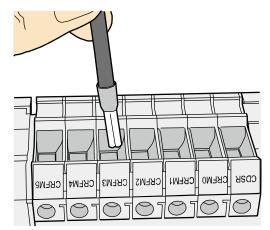
**Step 2** Insert the terminal into the jack vertically, and fasten the terminal by turning the matching screw in the clockwise direction, as shown in Figure 5-49.
