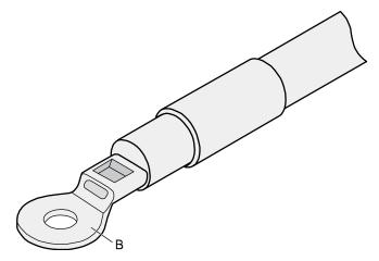
**Step 5** Push the heat shrink tubing (A) towards the connector until the tube covers the crimped part, and then heat the tube by using a heat gun, as shown in Figure 5-5.
