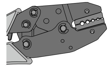
**Step 6** Hold the handles of the COAX crimping tools with one hand. Tighten the two fastening screws in the clockwise direction. Figure 5-77 and Figure 5-78shows the mould installed in the COAX crimping tools.
