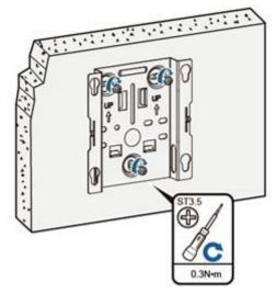
4. Align the mounting screws at the rear of the AP with the mounting holes on the sheet metal mounting bracket and then press the AP downwards to secure the AP on the bracket.
