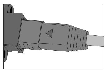
**Step 4** To disassemble an MPO fiber connector, hold the shell labeled "PULL" and remove the male connector, as shown in Figure 5-71.
