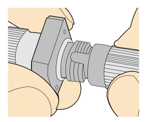
**Step 4** Fasten the locking nut in the clockwise direction and ensure that the connector is securely installed, as shown in Figure 5-60.
