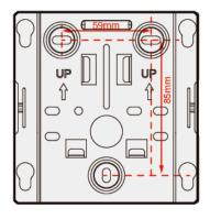
2. Use a 6 mm drill bit to drill 25 mm to 30 mm deep holes in the drilling positions. Hammer the expansion tubes into the holes until the expansion tubes are completely embedded into the wall.
