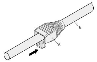
**Step 2** Remove a 30 mm (1.18 in.) long section of the jacket, cut off the nylon twine inside the jacket, and cut a no more than 5 mm (0.20 in.) cleft in the jacket, as shown in Figure 5-17.
