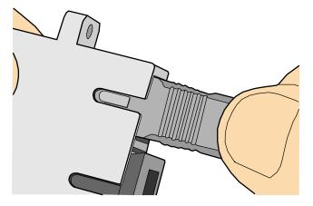
**Step 4** To disassemble an SC fiber connector, hold the shell of the connector (do not hold the fiber) and gently pull the connector in the direction vertical to the adapter. Unlock the male connector, and then separate it from the shell, as shown in Figure 5-68.
