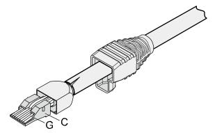
**Step 8** Put the connector body onto the wire holder and turn the metal shell by 90°, as shown in Figure 5-25.
