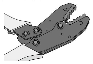
Step 3 Remove the mould from the COAX crimping tools, as shown in Figure 5-74.
