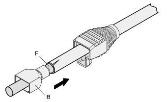
**Step 4** Fit the metal shell onto the twisted-pair cable until the shield layer is covered completely. Along the edge of the metal shell, cut off the aluminum foil shield layer and ensure that there is no surplus copper wire. The exposed twisted-pair cable is about 20 mm (0.79 in.) long, as shown in Figure 5-19.
