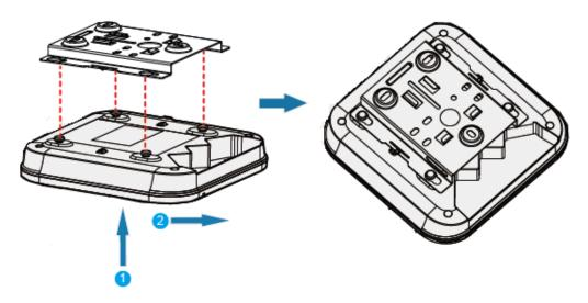
The screws provided for ceiling-mounting of APs are 30 mm long and can be used to fix an AP on a ceiling not thicker than 15 mm. To install APs on thicker ceilings, you need to purchase longer screws.
