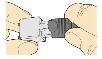
**Step 3** When you hear a click, the cable connector is completely inserted in the port. (The clip on the cable connector pops up to fix the connector in the port.) Pull the connector slightly and ensure that it is securely connected, as shown in Figure 5-52.
