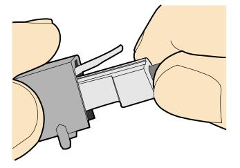
Figure 5-55 Feeding the male connector into the female unshielded connector
