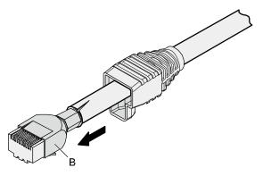
**Step 10** Push the jacket towards the metal shell until the metal shell is covered. This completes the assembly of one end of the cable, as shown in Figure 5-27.
