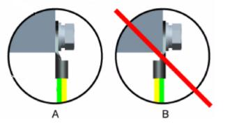
2. Place the spring washer and flat washer in turn, mount a matching screw, and fasten it clockwise, as shown in Figure 5-44.
