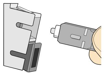
**Step 3** Feed the fiber connector into the female connector, with your fingers holding the shell of the fiber connector (not the pigtail). When you hear a click, the fiber connector is secured by the clips (internal parts, not illustrated in the figure). Pull the fiber connector gently. If the connector does not loosen, the installation is complete. See Figure 5-67.
