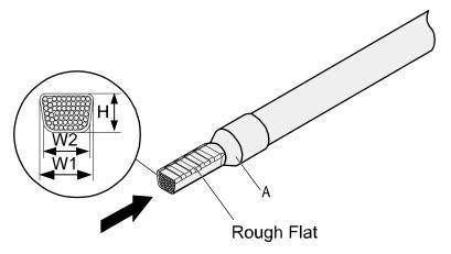
**Step 4** Check the maximum width of the tubular crimped terminal. The maximum width of a tubular crimped terminal is listed in Table 5-4.
