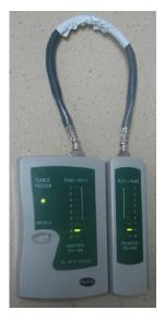
**Step 3** Gently shake the connector and repeat Step 2 to check whether the metal contact strips are in good contact with the core wires and Ethernet ports, as shown in Figure 5-40.
