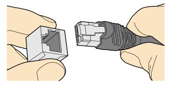
Step 2 Insert the male connector into the female connector, as shown in Figure 5-51.
