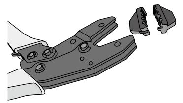
**Step 4** Place the mould to be installed into the jaw of the COAX crimping tools and align the screw holes, as shown in Figure 5-75.
