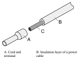
C. Conductor of a power cable
