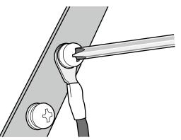
Figure 5-44 Installing two terminals back to back
