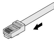
**Step 4** To complete the assembly of the other end, repeat Step 1 through Step 3.
