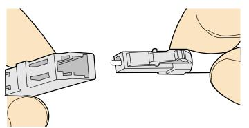
**Step 3** Align the male connector with the fiber adapter and gently push the male connector until it is completely seated in the fiber connector, as shown in Figure 5-63.
