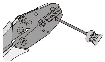
Figure 5-72 Loosening two fastening screws
