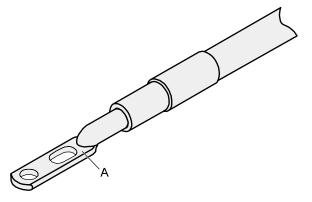
**Step 5** Push the heat shrink tubing towards the connector until the tube covers the crimped part, and then heat the tube by using a heat gun, as shown in Figure 5-10.
