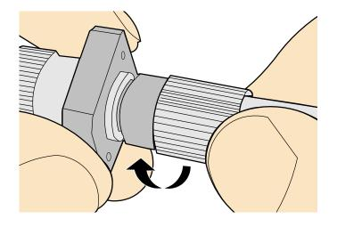
**Step 5** To disassemble an FC fiber connector, loosen the locking nut counterclockwise, and gently pull the male connector, as shown in Figure 5-61.
