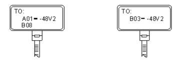
Label on the loaded cabinet side (indicating he position of the cable on the power distribution box)
