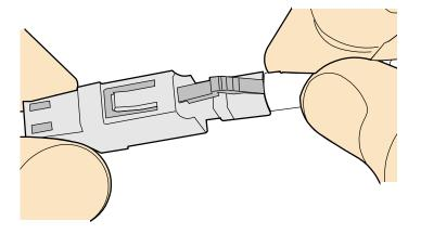
Step 4 A clicking sound indicates that the male connector is locked, as shown in Figure 5-64.
