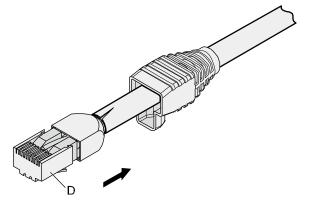
**Step 9** Push the metal shell towards the connector body until the wire holder and the connector body are engaged completely. Crimp the connector, as shown in Figure 5-26.
