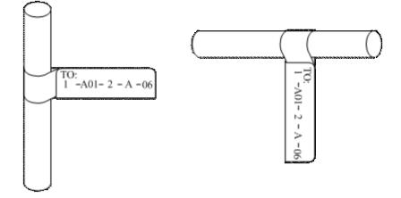
• Procedure for attaching labels Figure 5-86 shows the methods and procedures for attaching labels.
