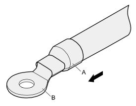
**NOTICE** Stop heating the shrink tubing when the connector is securely locked in the shrink tubing. Do
