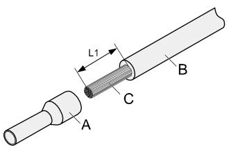
Table 5-3 Mapping between the cross-sectional area of the conductor and the value of L1
