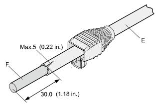
Step 3 Fit the metal shell onto the twisted-pair cable. The shield layer is covered by the metal shell, as shown in Figure 5-18.
