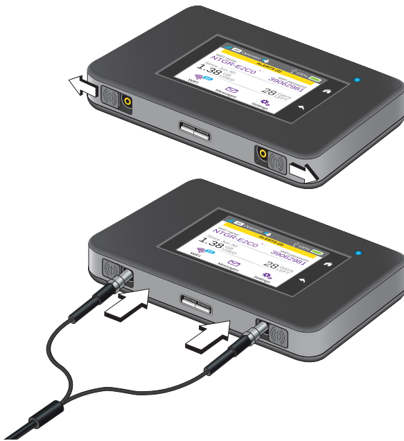
Figure 4. External antennas with TS-9 connectors
