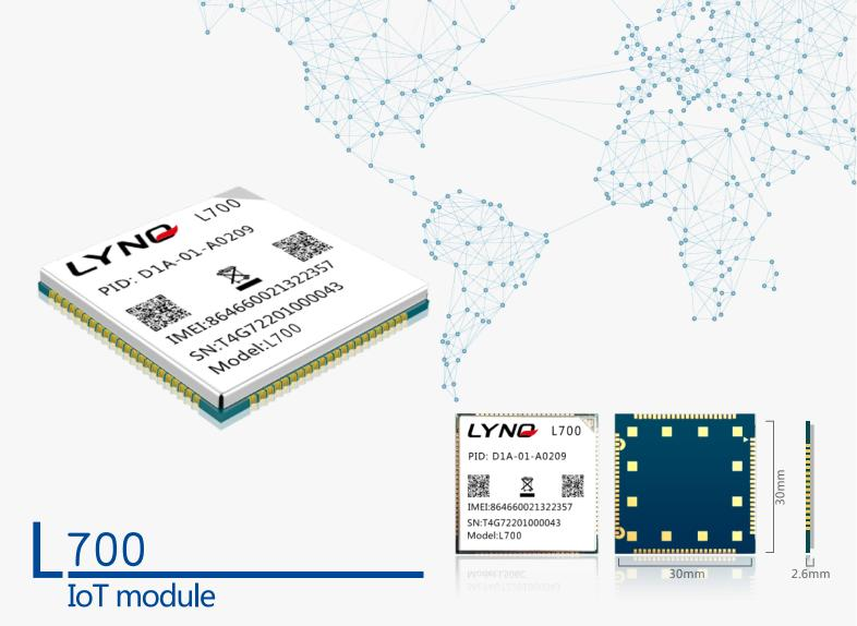
L700 is a IoT module with excellent reliability, occupied small area base on industry-leading Qualcomm MDM9206 platform, It supports LTE CAT-M1 and CAT-NB1,GSM/GPRS/EDGE.
