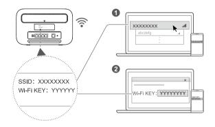
Once the router has connected to a mobile data network, you can connect your computer or mobile phone to the router's Wi-Fi network to access the Internet. Please refer to the label on the bottom of the router for the default wireless network name (SSID) and password (Wi-Fi KEY).
