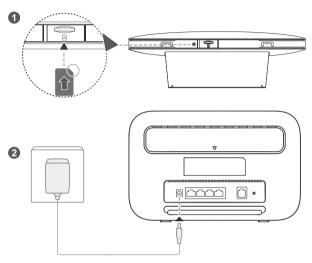
Insert a micro-SIM card into the micro-SIM card slot as shown in the preceding diagram and then connect the power adapter to the B612 router. The router will turn on automatically and search for available mobile networks.
