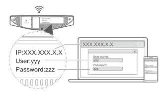
You can configure the router using the web-based management page. Please refer to the label on the bottom of the router for the default IP address, user name, and password.
