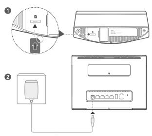
Insert a micro-SIM card into the micro-SIM card slot as shown in the preceding diagram and then connect the power adapter to the B525 router. The router will turn on automatically and search for available mobile networks.
