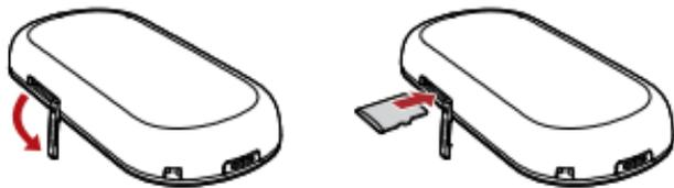
2. After inserting the microSD card completely, attach the rubber cap.
