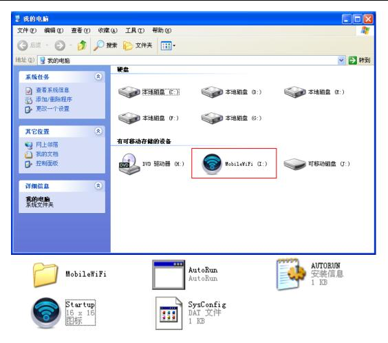
4. If the drive path MobileWiFi not showing up, make sure there is no damage on USB cable and no contamination at PC USB connectors. Try to re-plug in USB connectors (both end of USB cable) to E5331 and computer again.
